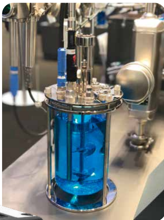
bio-Optic connected to RamanRxn probe installed in a bioreactor
